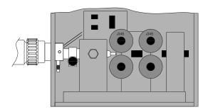
6. Disconnect the welding gun from the adapter plug and slide the supplied plastic insulating flange over the adapter and up to the outer panel-face of the feeder. Position the flange so that the opening for the gas hose is located in line with the gas nipple of the adapter block (normally down position).
