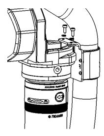
Lay the extraction hose along the robot arm and between the halves of the hose-management clamp. Keep the clamp as far forward on the robot arm as practical while maintaining a sufficient service loop in the front to allow the robot complete range of motion without excessive pulling, twisting or binding of the extraction hose.
