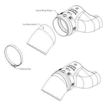
Note: if the suction boot does not appear to be more-or-less concentric with the swanneck it may be due to the boot being installed backwards. Try placing the opposite end of the boot onto the mounting ring. If the boot is still not concentric, try to skew the boot on the ring as necessary before clamping.
