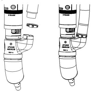
Align the hose guide and aluminum bracket over the hose in close proximity to the hardware holes on the robot arm. Tighten the screws to secure the extraction hose to the hose guide.
