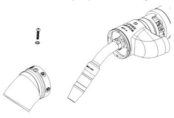
• Line the screw up with the curvature of the swanneck; it should be directly over top of the locking tab.
