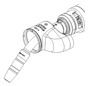
• Holding the housing in place, slide the suction boot coupler ring over the swanneck and snap into position on the housing.
