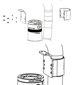
Mount the bracket to the robot arm. The hose can be pulled up or down in the hose guide for final adjustment. Ensure the hose is in a "neutral" position that is not pushing or pulling on the main housing.
