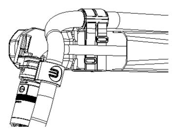
• Secure the clamp by cinching the elastic hook-n-loop straps through the clamp and around the robot arm.
