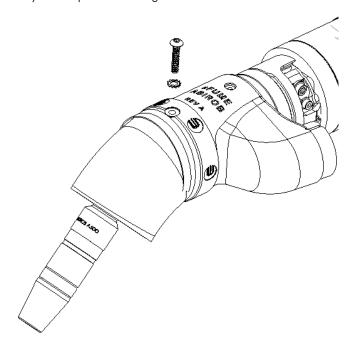
• Tighten the screw, making sure it is aligned with the hole in the locking tab, until the washer teeth engage.
