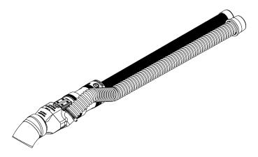
Lay the extraction hose along the robot arm and between the halves of the hose-management clamp. Keep the clamp as far forward on the robot arm as practical while maintaining a sufficient service loop in the front to allow the robot complete range of motion without excessive pulling, twisting or binding of the extraction hose. Secure the clamp by cinching the elastic hook-n-loop straps through the clamp and around the robot arm. The clamp should not be able to move easily under the straps.
