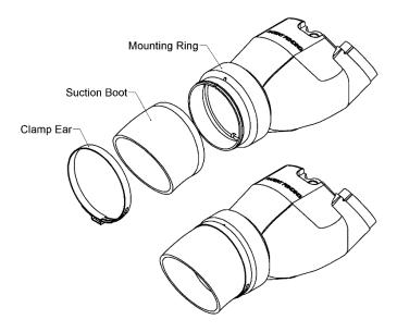
Note: If the suction boot does not appear to be more-or-less concentric with the swanneck it may be due to the boot being installed backwards. Try placing the opposite end of the boot onto the mounting ring. If the boot is still not concentric, try to skew the boot on the ring as necessary before clamping.
